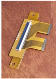
1. Obtain the adaptor for your PCAP sensor flex cable.
