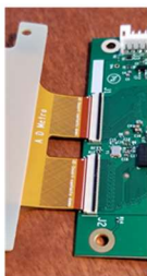
5. Insert the two ends of the flex tail fully into the two connectors.
