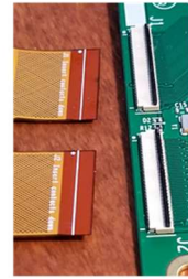
4. Gently rotate the black latches up to open the connectors.
