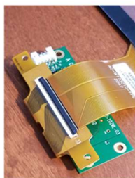
13. Fold down and close the black latch of the connector.
