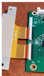
6. Fold the black connector latches down to close the connectors.
