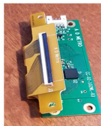
7. Bend (don't crease) the adaptor's flex cable so that the two adaptor board holes roughly align with the closer two controller board holes.
