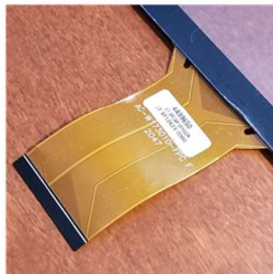
10. Orient the flex tail metal contacts facing down.
