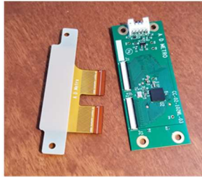
2. Turn the adaptor upside-down, ready to connect to a PCAP controller.
