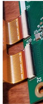
YES!! Gentle bend in flex cable eliminates stress on connectors.
