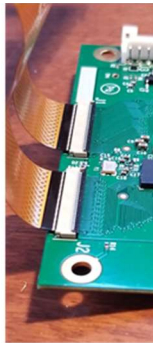
NO!! Unwanted stress applied to connectors from upward-pulling flex cable.
